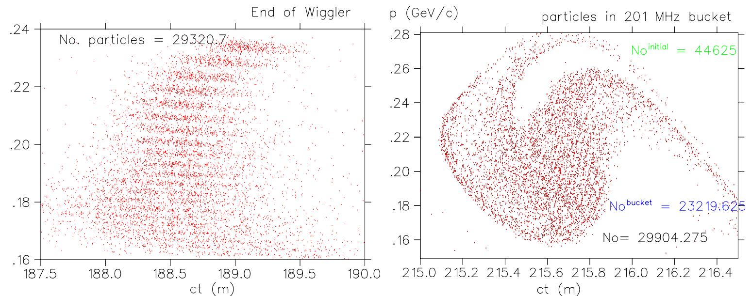
Long phase space at the end of the wiggler (LEFT); at the end of the bucket formation section (RIGHT).
