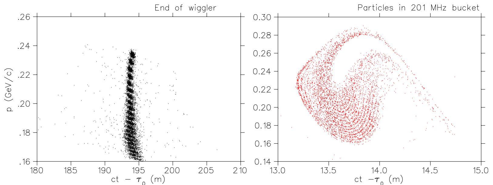
Long phase space at the end of the wiggler (LEFT); at the end of the bucket formation section (RIGHT).
