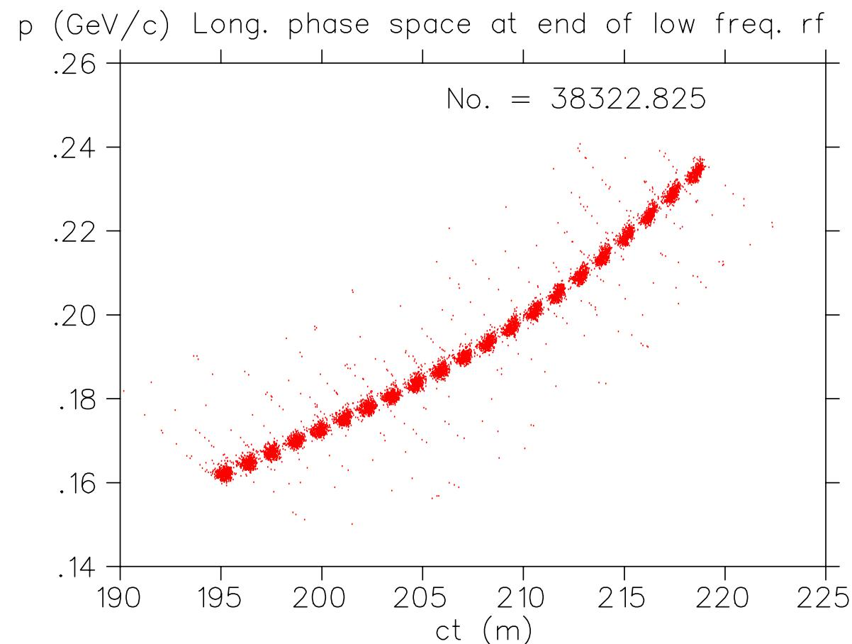
Notice that the lower energy particles are ahead in the bunch train;  $L_{train} \approx 30 m.$
