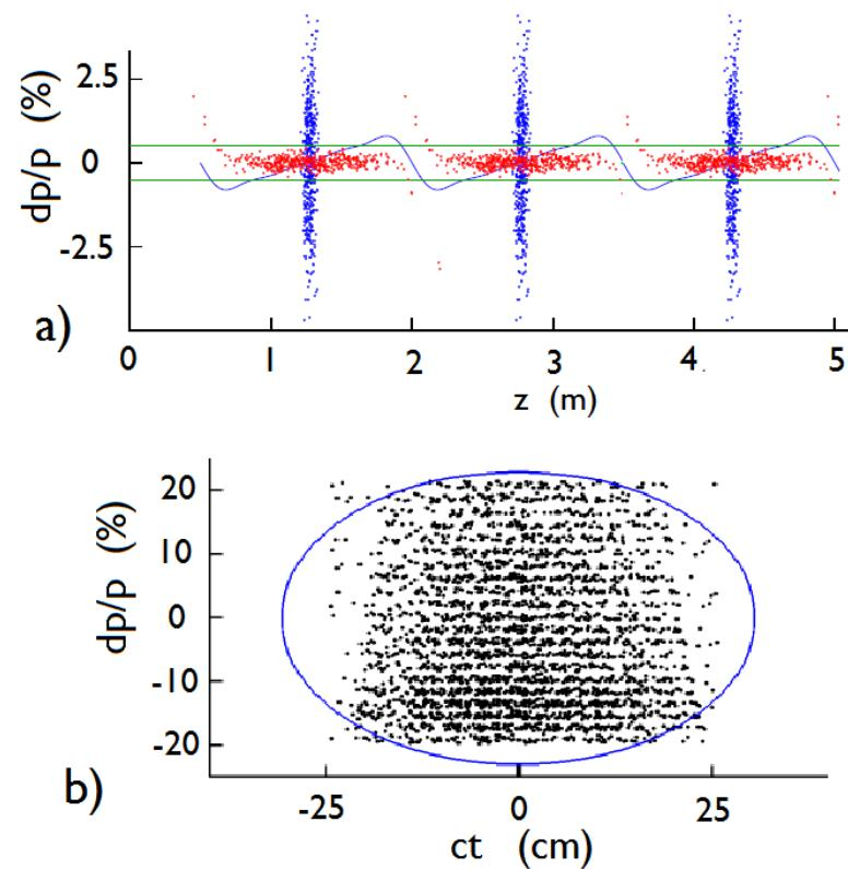
1-D Simulation: a) before (blue) and after 1<sup>st</sup> rotation (red);
