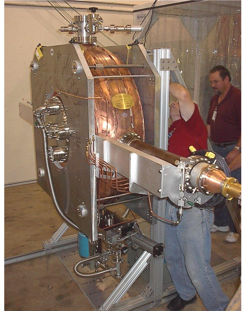
The 201-MHz cavity at MTA
