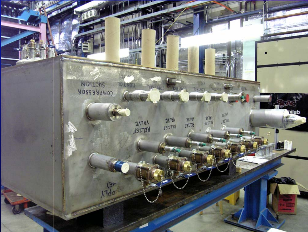
Completed Valve Box
