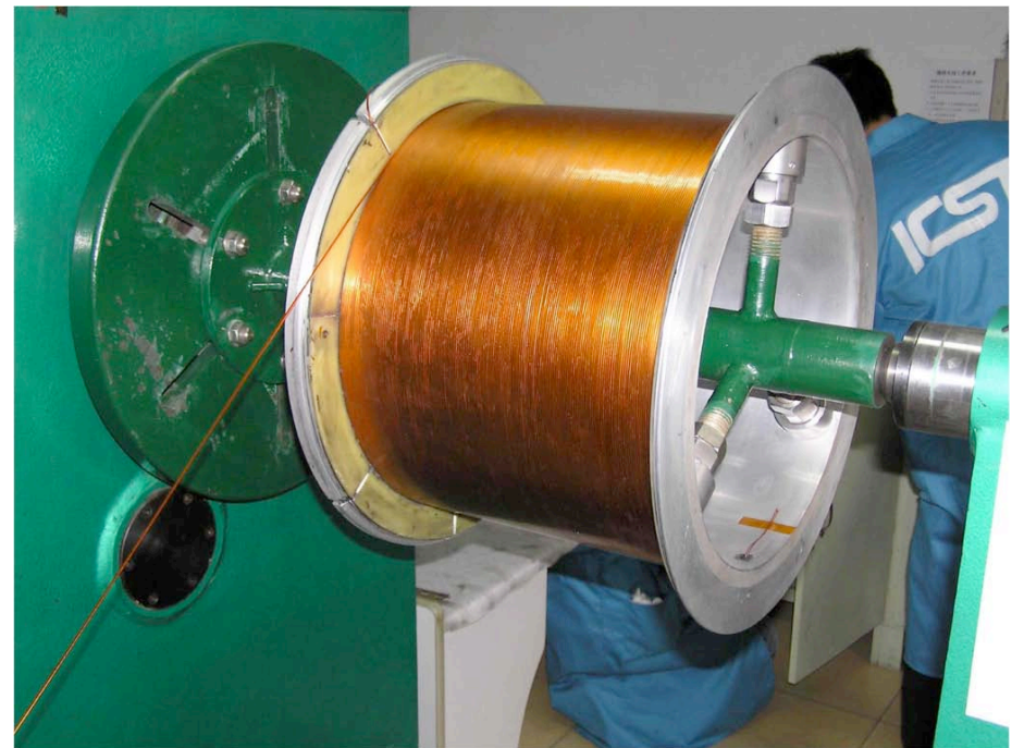
Application of fiberglass for winding of second layer
