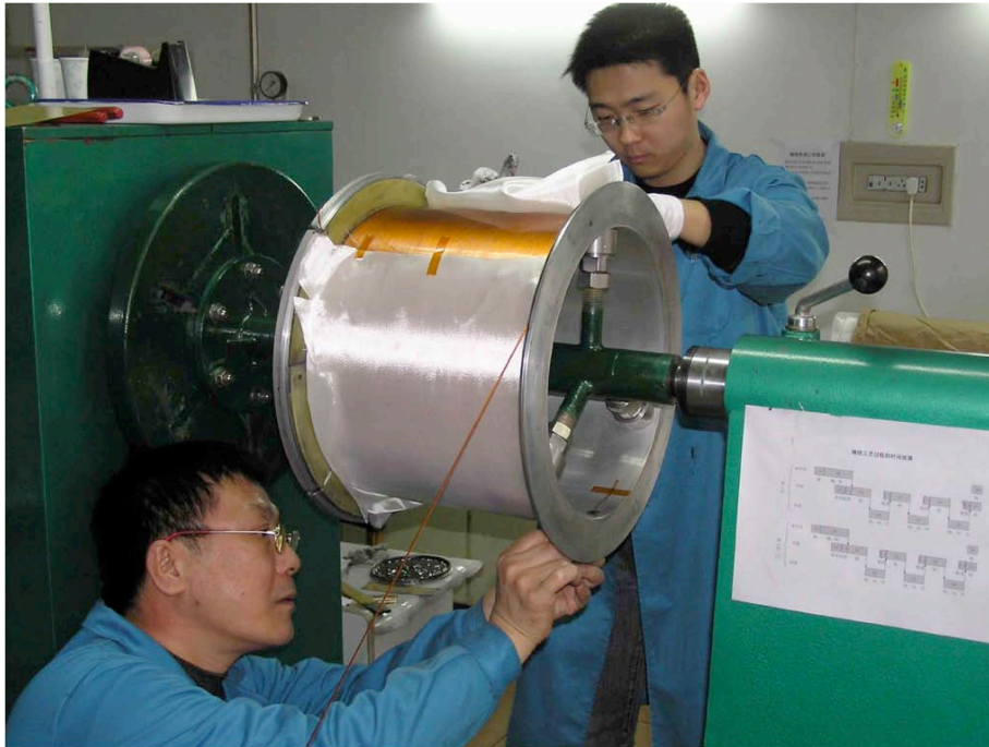
Application of fiberglass for winding of second layer
