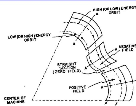
FIG. 2. Plan view of radial-sector magnets.
