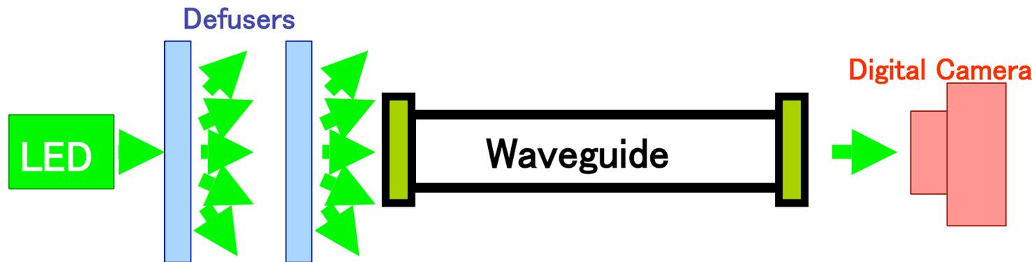
LED : Wave length=525nm(3HF : Wave length=520nm)
