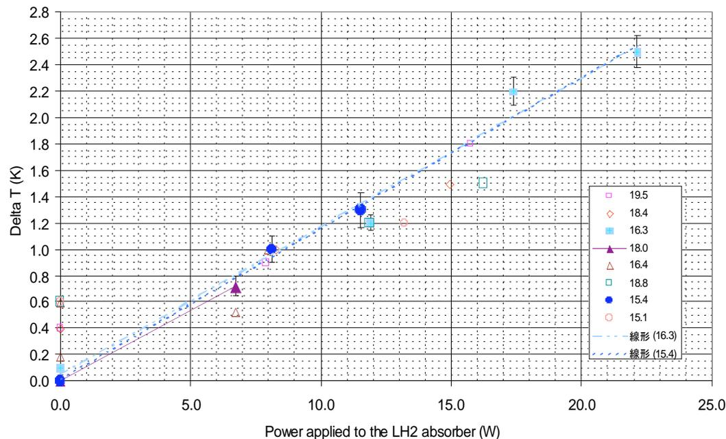
Temperature gradient (TC-106-H - TC-110-H) versus applied heat for several LH2 absorber bath temperatures.
