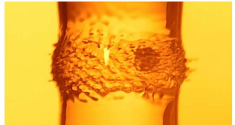
Water jet ripples generated by a 8 mJ Laser cavitation bubble
