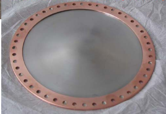
Curved Be window for the 805-MHz pillbox cavity
