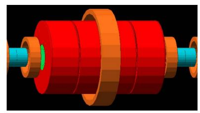
Cooling 1/2-cell: two absorbers (blue), three coils (brown), two focusing and one coupling, and four rf cavities (red)
