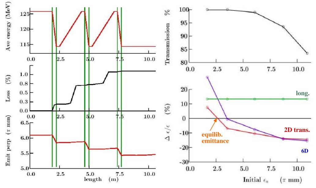
→ ≈10% transverse emittance reduction, measurable to 0.1% (abs.) given precise spectrometer, clean beam, and efficient, redundant particle ID
