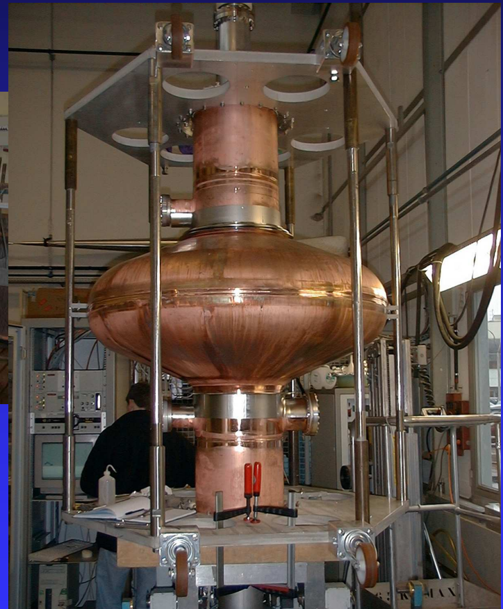
Magnetron Nb film (1-2 \mu\text{m} ) sputtering
