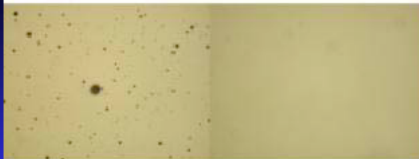
SEM pictures of film surface with/without macro particle filter
