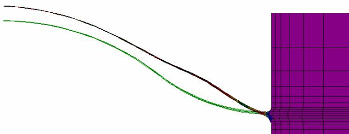
Behavior of window under an incremental **internal** pressure until burst
