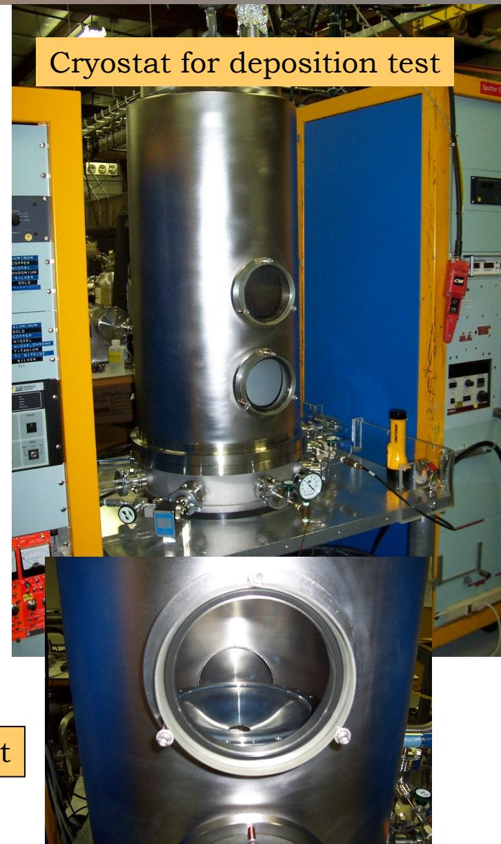
Broken window in deposition test
