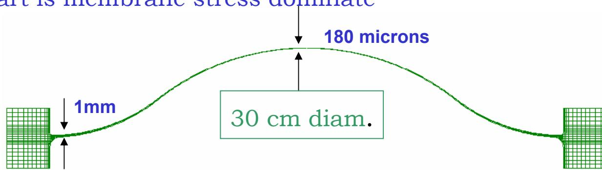
The current window FEA analyses show that the shape scales can use same analysis for different diameters of same profile!
