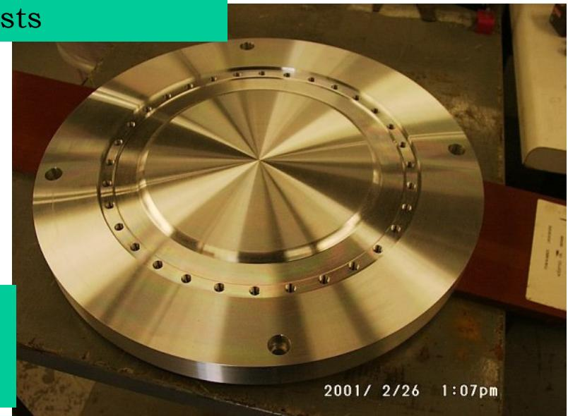
Flange/window unit machined from aluminum piece (torispherical 30 cm diam)
