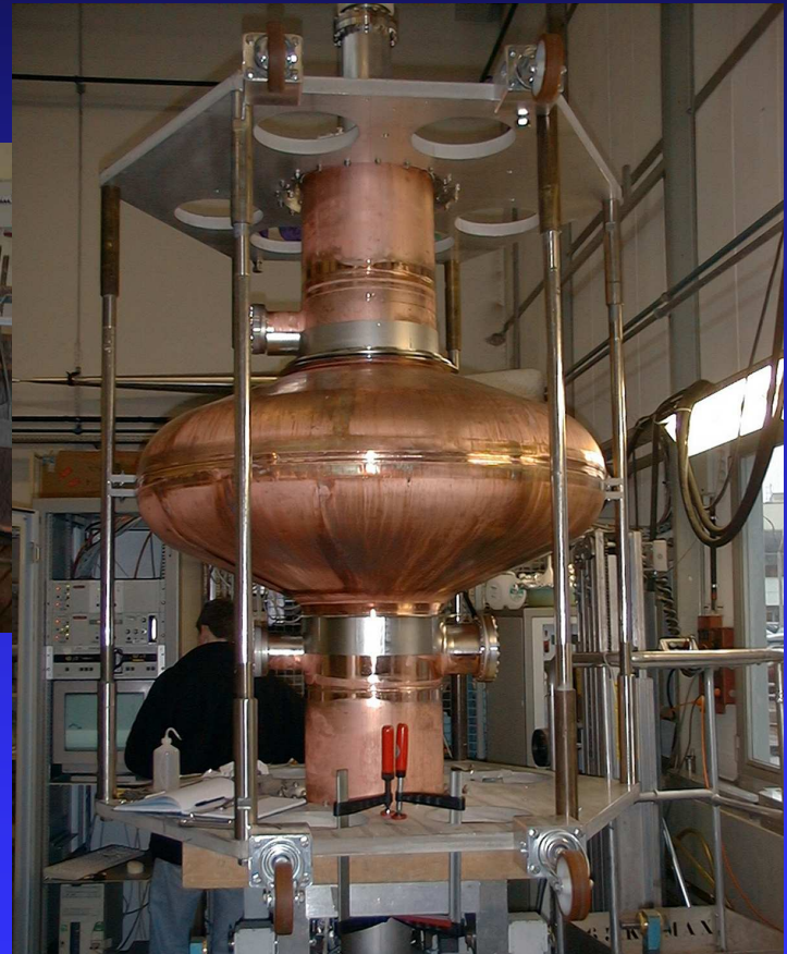
Magnetron Nb film (1-2 \mu\text{m} ) sputtering
