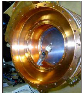
Tested Be-Windows for RF Cavities – LBNL
