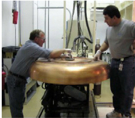
201 MHz half-shell ebeam welding of Stiffening – JLab
