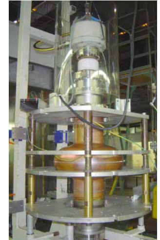
500 MHz Cavity for sputtering studies – Cornell
