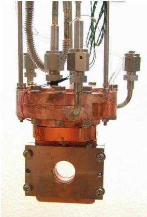
Calibration of LH2 Level Sensor – KEK
