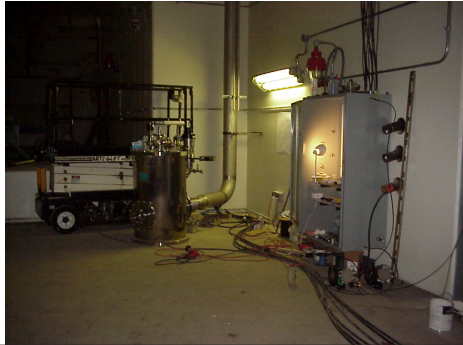
LH2 Absorber Cryostat installed in MTA FNAL/KEK
