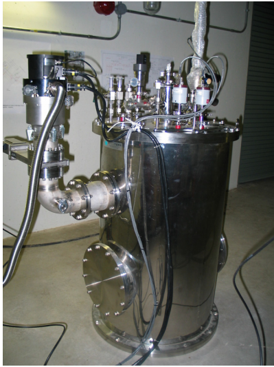
LH2 Absorber Cryostat – KEK
