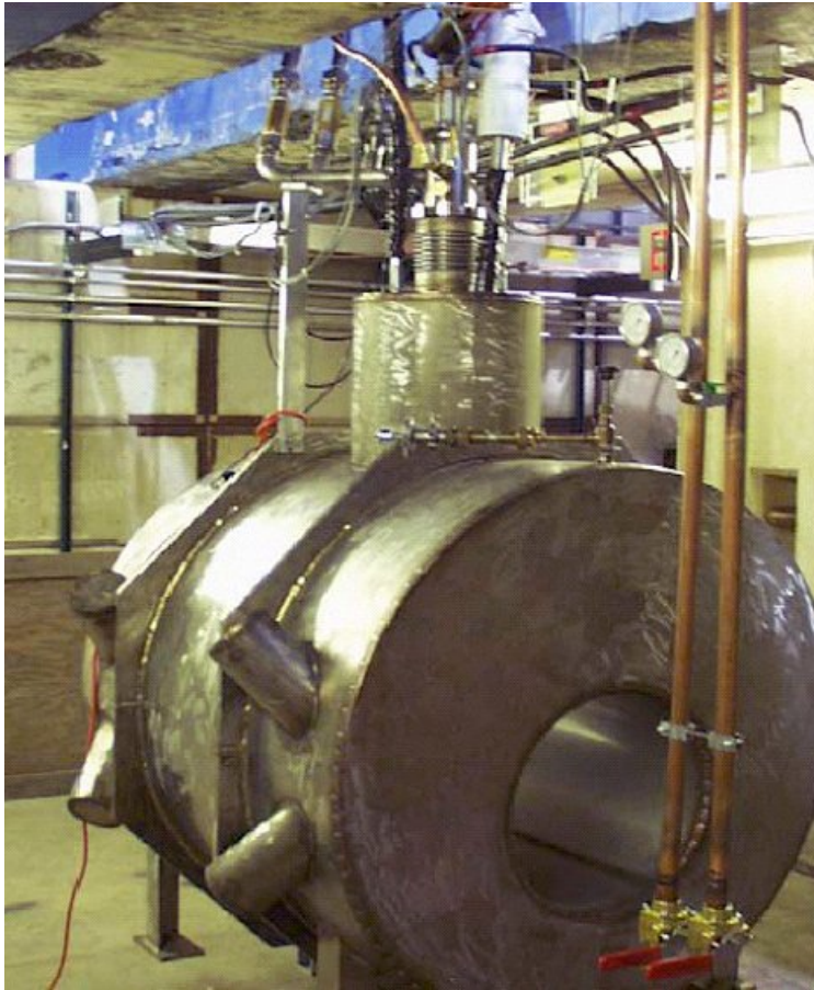
Lab G RF Test Cave showing 5T SC Magnet 44 cm bore R.I.P.
