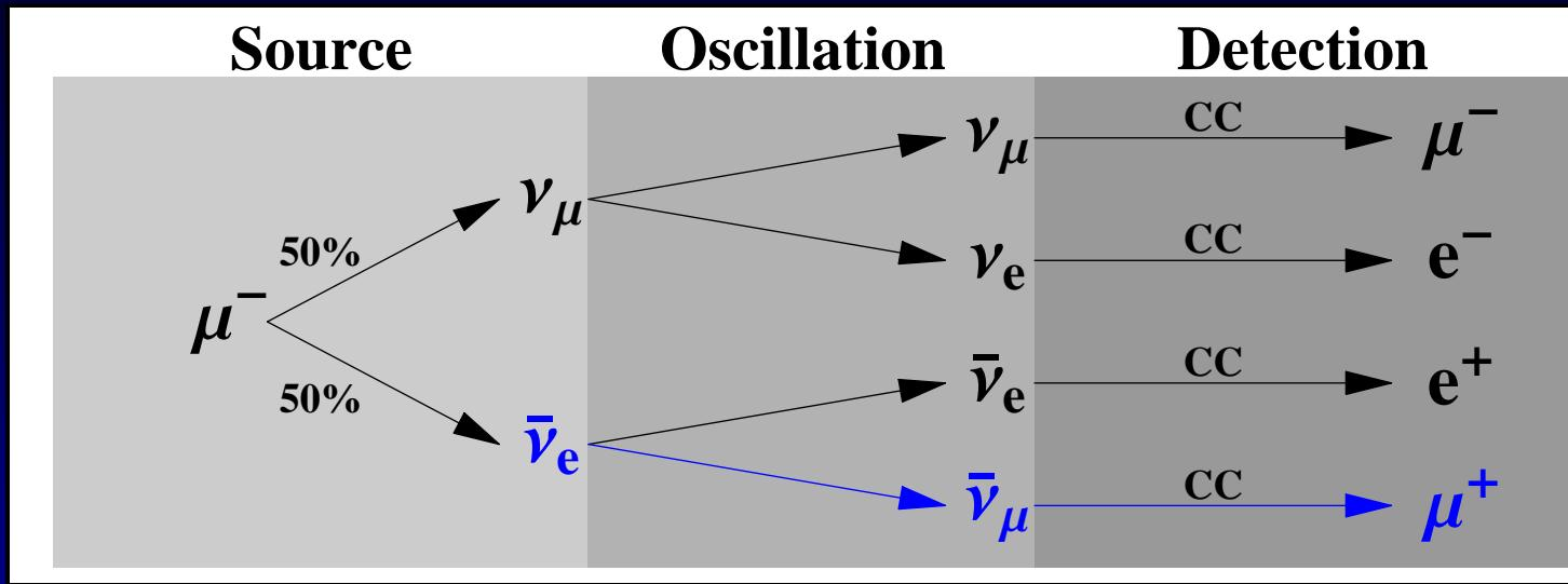
This requires a detector which can distinguish  $\mu^+$  from  $\mu^- \Rightarrow$  magnetic field of around 1T
