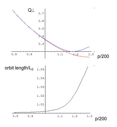
Transverse dynamic aperture obtained by tracking particles 25 periods w/o stochastics and with initial conditions J1=J2, J3=0,  $\psi$ 1= $\psi$ 2=0:
