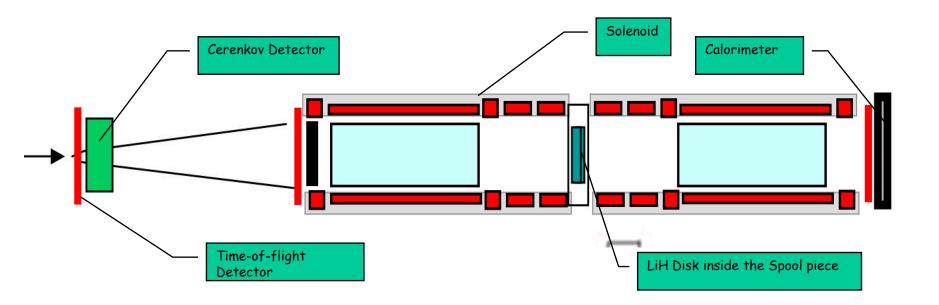
Produce 50 cm Ø X 6.5 cm thick disk for MICE for first "cooling" measurment
