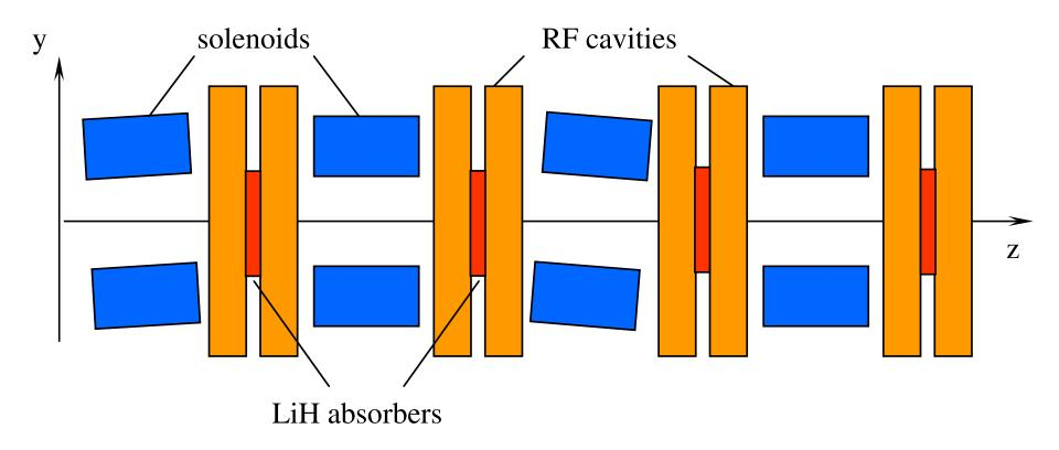
Cell length =3.2 m, solenoid inner radius = 40cm, Bmax=2.4 T at p=100MeV/c HPRF cavities  $2\times16$ cm long, E=25MV/m, GH2 fill with density 10% of LH2 Emittance decrement 1/25m, equilibrium emittances ~1.5  $\pi$ ·mm
