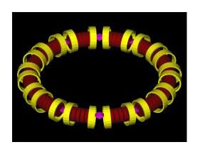
$P_{ref} = 201 - 204 \text{ MeV}$  (25th harmonic) RF grad=11.451 - 12.835 MV/mRF freq=201.25 MHzCells=12Circumference=33 mCoil Tilt=3 deg
