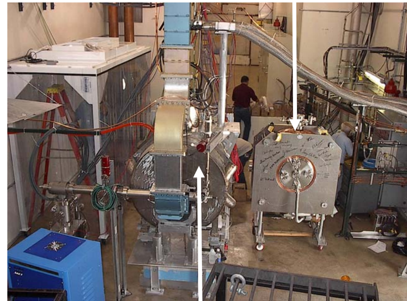
5-T solenoid + 805-MHz cavity
