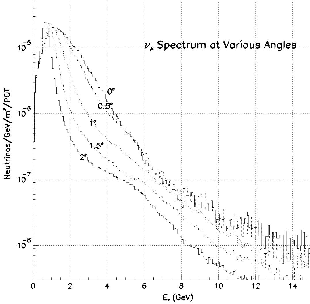
Wide band neutrino beam at 1 km designed for the E889 experiment at BNL at various angles.
