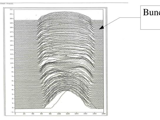
Bunch Dilution using VHF cavity
