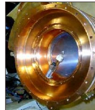
Tested Be-Windows for RF Cavities – LBNL
