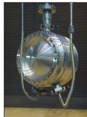
Liq.H Absorber – KEK To be tested at FNAL
