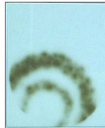
Dark current ring measurements on glass plate – ANL/FNAL/IIT
