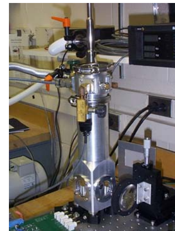
Bolometer detectors for Window Beam profile – cryogenic setup– U. Chicago
