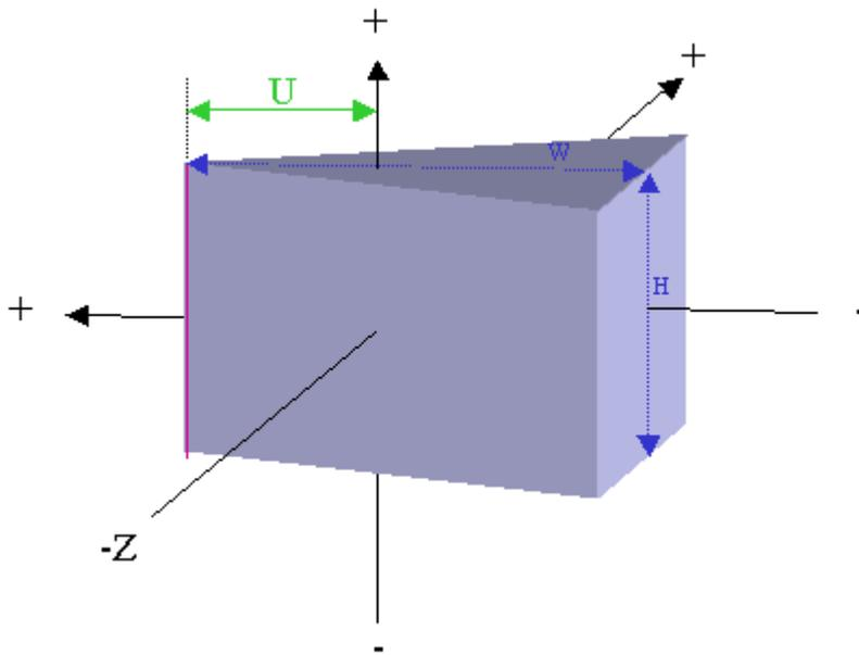
The wedge geometry can accept a second MTAG parameter in the SREGION construct. The first material refers to the interior of the wedge. The second material, if present, refers to the exterior of the wedge. If a second MTAG parameter is not present, vacuum is assumed.
