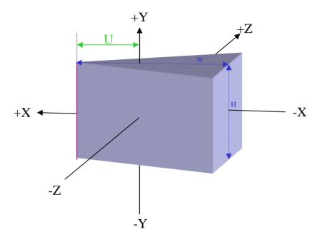
The wedge may be translated in the X direction by adjusting parameter U. Setting U>0 moves the wedge a distance U in the +X direction. For example, setting U = W/2 centers the wedge in the X direction. The wedge retains its symmetry about the XY plane Z=0 and the XZ plane Y=0.
