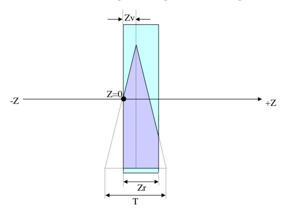
This wedge does not fit within its region. Zv < T/2 and Zr < Zv + T/2. The material outside the region boundaries is not seen when particles are propagated through the wedge. There are probably few cases in which this sort of truncation is useful.
