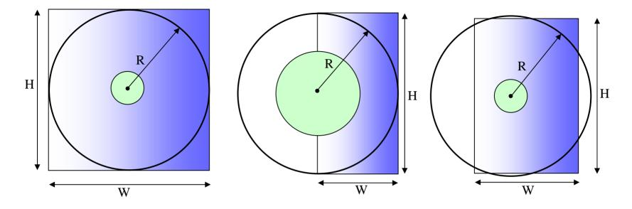
It is possible (though seldom useful) to define a wedge within a radial subregion having non-zero inner radius – an annular subregion. In such cases, particles passing through the wedge inside the inner radius of the subregion (green) do not encounter any of the wedge's absorber.
