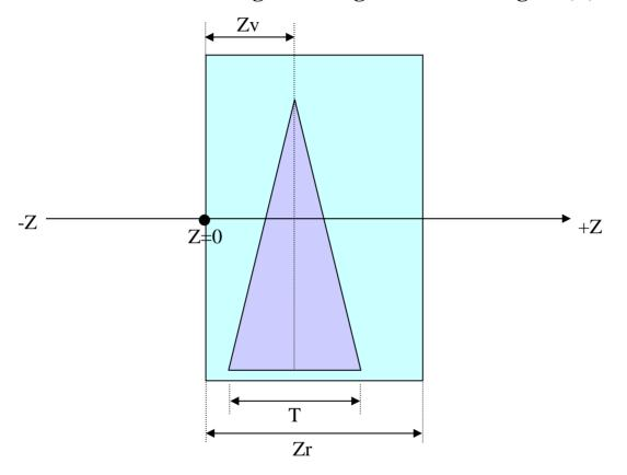
By setting Zv > 0, the wedge is translated in the +Z direction. If Zv > T/2 and Zr > Zv + T/2, then the entire wedge is within its region in the Z direction. Recall that  $T = 2W \tan(A/2)$ . It is perfectly normal to define wedges that do not fill their region in Z; the region's material outside the wedge is assumed to be vacuum.
