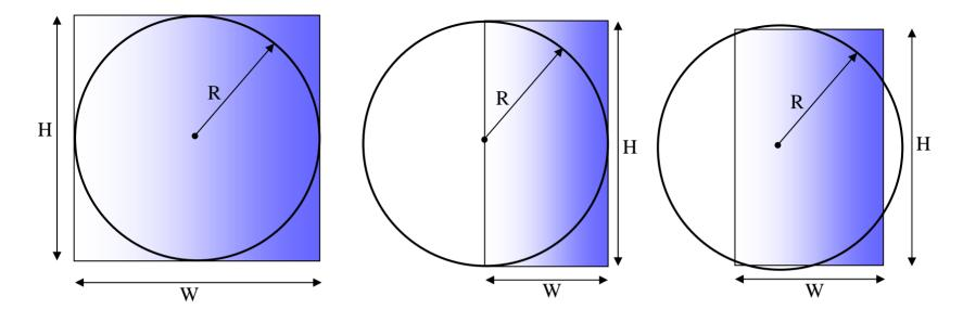
Here we view a wedge from the beam's perspective. The Z axis is in the center of a radial subregion (circle) of radius R. The wedge presents a cross-section of width W and height H to the incoming beam. In all three examples, PHI=0; the gradient of increasing thickness (blueness) lies in the -X (right) direction. (In these examples we presume that the entire wedge lies within the Z-boundaries of its region, and that the subregion has an inner radius of zero.)
