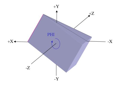
Next, the wedge may be rotated about the Z axis by an angle PHI. Looking in the beam direction (+Z), clockwise rotations are positive. In the illustration above, PHI is about +30 degrees. Setting PHI = +90 degrees would place the vertex line horizontal at Y=U, with the Z-thickness gradient lying in the –Y direction. The wedge retains its symmetry about the XY plane Z=0, but in general the symmetry about the XZ plane Y=0 is broken by the rotation.
