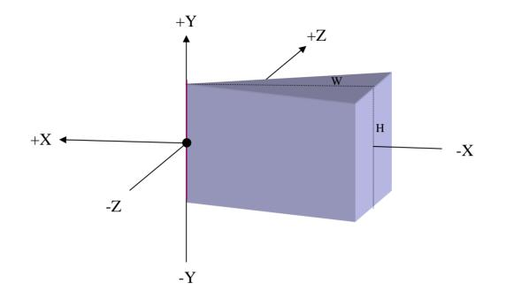
The wedge is initially oriented as shown. The vertex line of the wedge lies along the Y axis, extending from Y=-H/2 to Y=+H/2. The wedge is symmetric about the XY plane Z=0 and symmetric about the XZ plane Y=0. The wedge's Z-thickness gradient lies in the -X direction.
