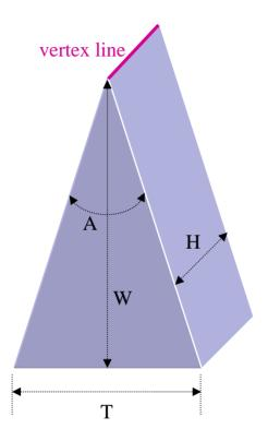
We begin by defining the size and shape of the wedge: The triangular sides of the wedge are isosceles triangles. The base-to-vertex distance is W The full angle at the vertex is A The side-to-side length of the wedge is H The vertex line of the wedge extends from one side's vertex to the other, as shown. The maximum thickness (T) of the wedge = 2W tan(A/2)
